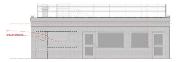
The rear of the building will have a staircase leading to the rooftop deck. The rooftop deck will be surrounded with posts and cables.
