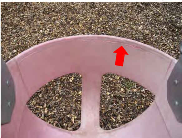
Bucket seat is cracking
