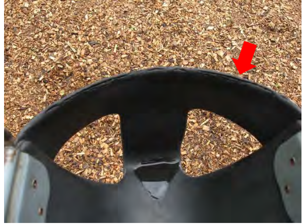
The bucket swing is cracking
