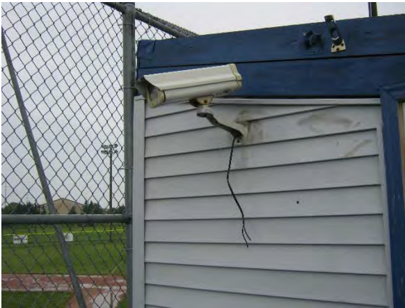
Damaged security camera at press box
