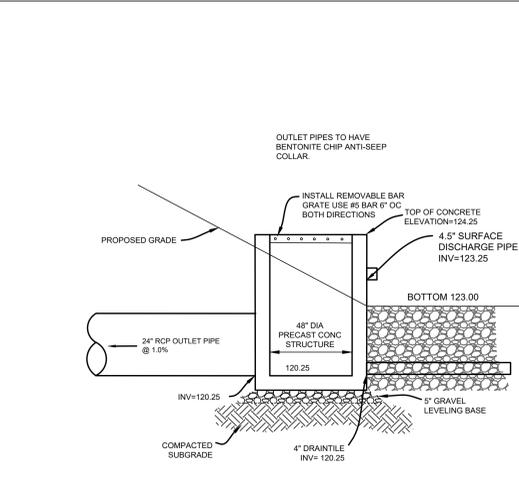
BIORETENTION OUTLET DETAIL
