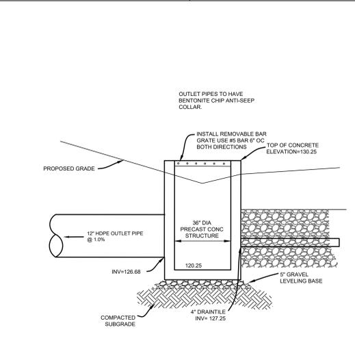
BIOSWALE OUTLET DETAIL
