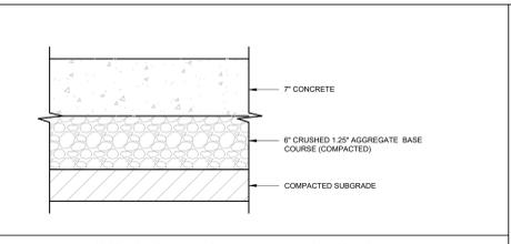
CONCRETE PAVEMENT SECTION
