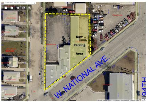
May site plan - The prior plan include changing the gradient of the property to match the east to the west. In other words, base material fill/soil will be added to increase the new parking area pavement surface to match the existing level of pavement at the west side of the site (9440 W. National Ave.). The fill then being graded to slope/drain from north to south. A retaining wall was proposed on the east side of the site, abutting the commercial property to the east.
