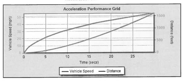
Acceleration Performance: TIME TO ACCELERATE ON A GRADE TO 55.0 (MPH) IS 29.97 (SECS)
