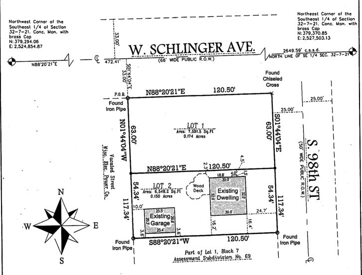
DENOTES SET 3/4" X 18" LONG IRON REBAR WEIGHING A MINIMUM OF 1.13 LBS PER LINEAL FOOT.
