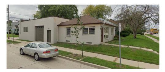
The proposal before Plan Commission is to add a second story to the existing building. Construction materials include corrugated metal siding on the second floor and new wood siding over the existing first floor. The roof will be made of new wood fascia boards.
