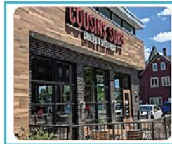
i. Using enduring materials like brick masonry, decorative concrete (in this example stylized as wood), and metal features ensures a building will age well and enhances the community's image.
