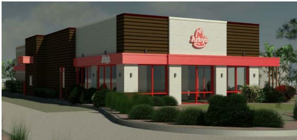
All four facades of the building will be updated with a more modern look. For the northern (front) half of the building, the existing metal coping, lighting, and red canopies will be removed. Thin brick (white & sable) and LP Smartsiding (brown) will be added on top of the existing masonry. Updated lighting fixtures and new metal canopies (red) will also be added.
