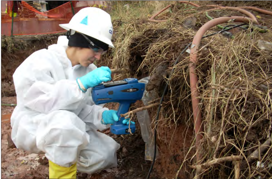
Field-screening of soils at an industrial remediation site
