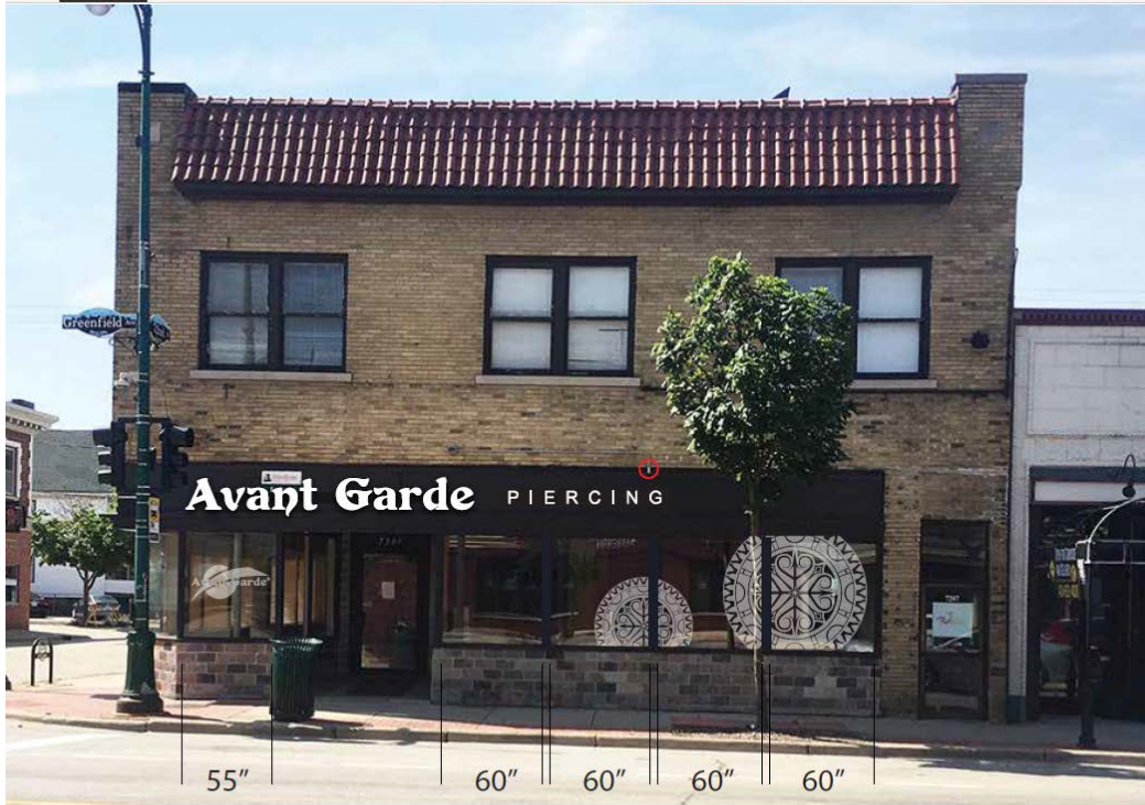
3M vinyl Frosted Crystal 7725E-324 on 1st surface (outside window)
