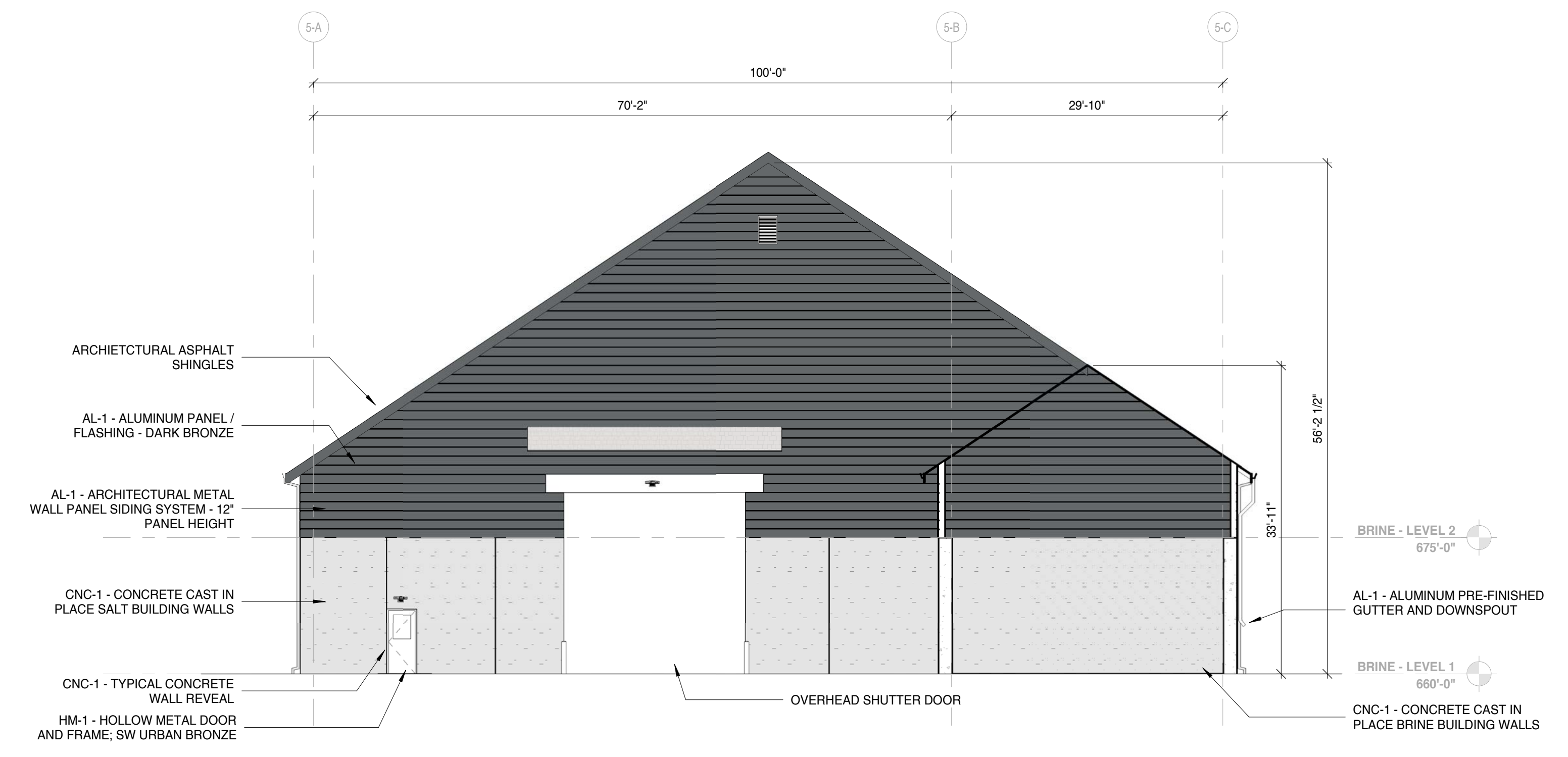
4 ELEVATION - BUILDING 05 - WEST 3/32" = 1'-0"
