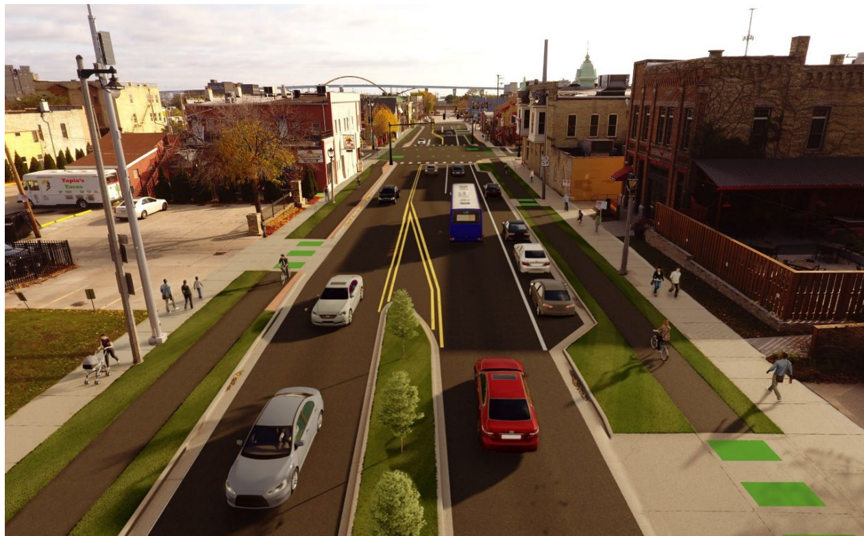
STH 59 will be transformed further East in Milwaukee with wider sidewalks, protected bike lanes, greening, and traffic calming (Source: WI Bike Fed)
