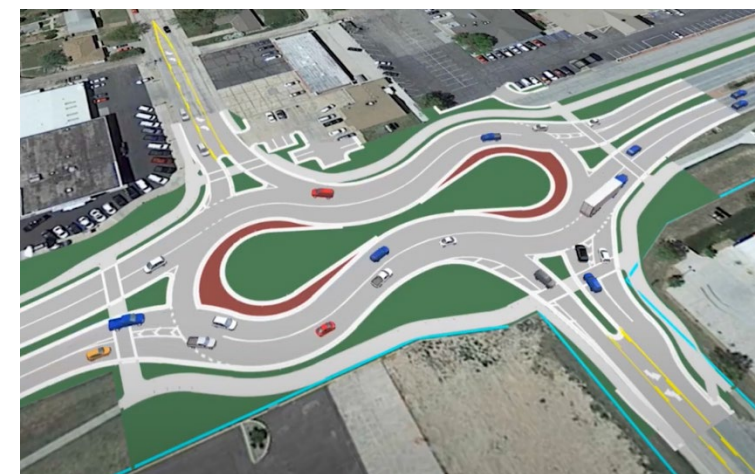
Designs like this "peanut" round-a-bout could be used to improve safety and traffic flow at intersections such as 84th and National
