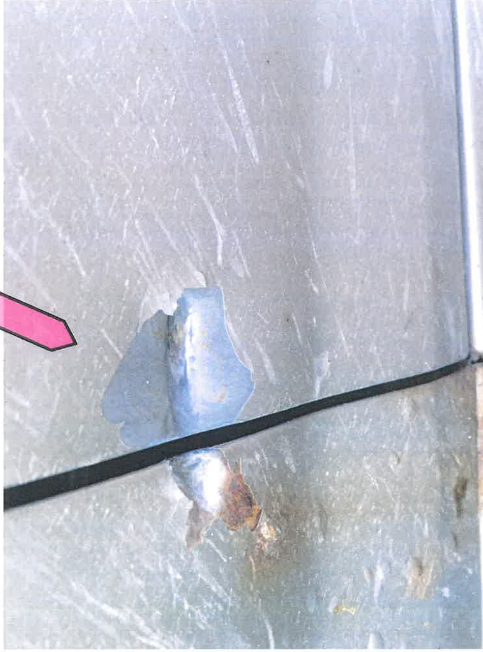
Drivers Side near front tire on drivers door - Bullet Ricochet #1
