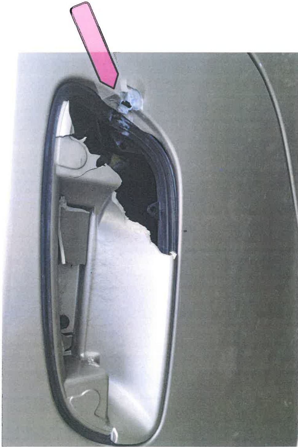
Drivers Side Rear door - bullet hole and broken handle view #2
