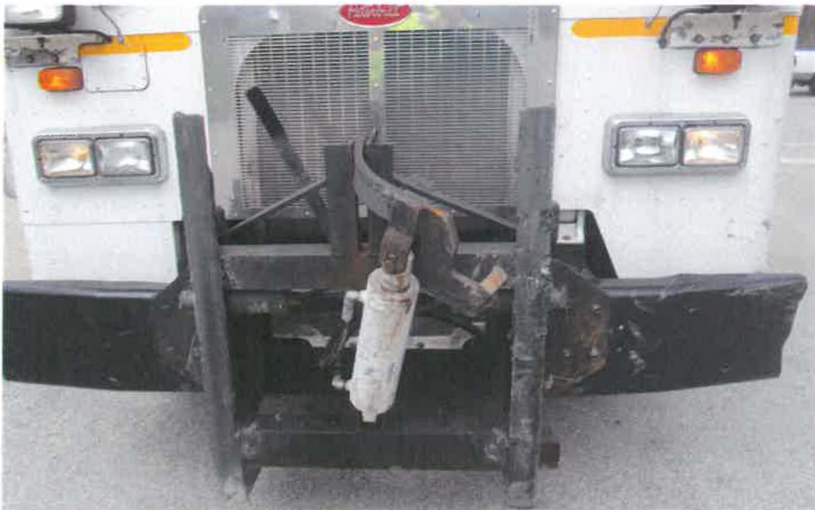
Damage to the front of West Allis's garbage truck due to the collision.
