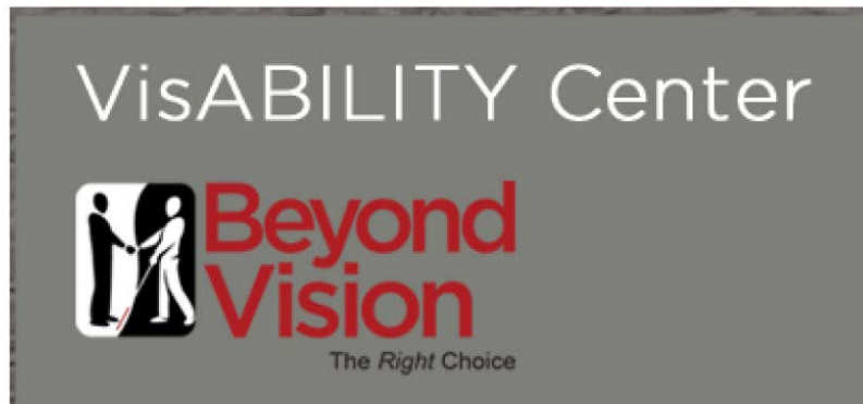
350' x 160" Flat Metal Painted Panel Backer 290" x 125" Individual Flush Mounted Letters/Logo to building facade Internally Illuminated Dimensional Channel Letters/Module White Acrylic Face (with vinyl) / Trim Cap / White Returns - White LED lighting inside each module
