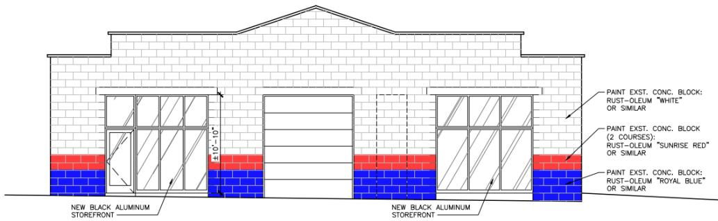
The submitted architectural plans largely mirror the changes proposed in the project's floor plans. The western exterior elevation marks the new storefront entryway to the workshop and removal of the old customer service entryway. Notably, the building will be repainted in rust-oleum white, with sunrise red and royal blue striping surrounding the lower portion of the building.
