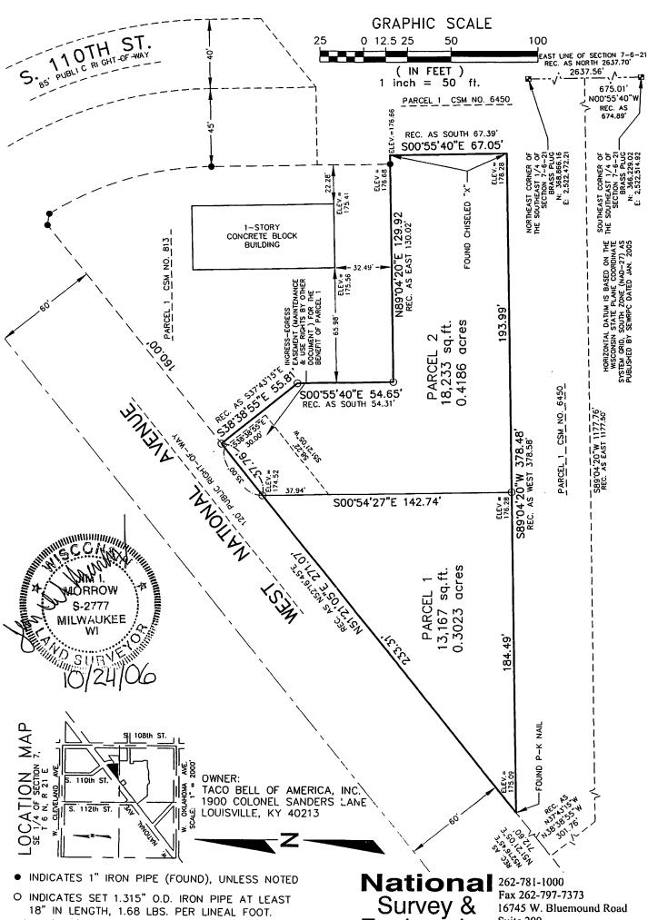
18" IN LENGTH, 1.68 LBS. PER LINEAL FOOT. ALL DIMENSIONS SHOWN ARE MEASURED TO THE NEAREST HUNDREDTH OF A FOOT.
