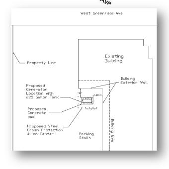
The City Hall generator has been used as a general guide/example for Allis Care center's project. Allis Care center will install a concrete pad upon which the new generator will be placed. A new pvc or comparable decorative screen fence will hide the generartor and in addition a curbed landscaping island will further protect and screen the perimeter of the new feature.
