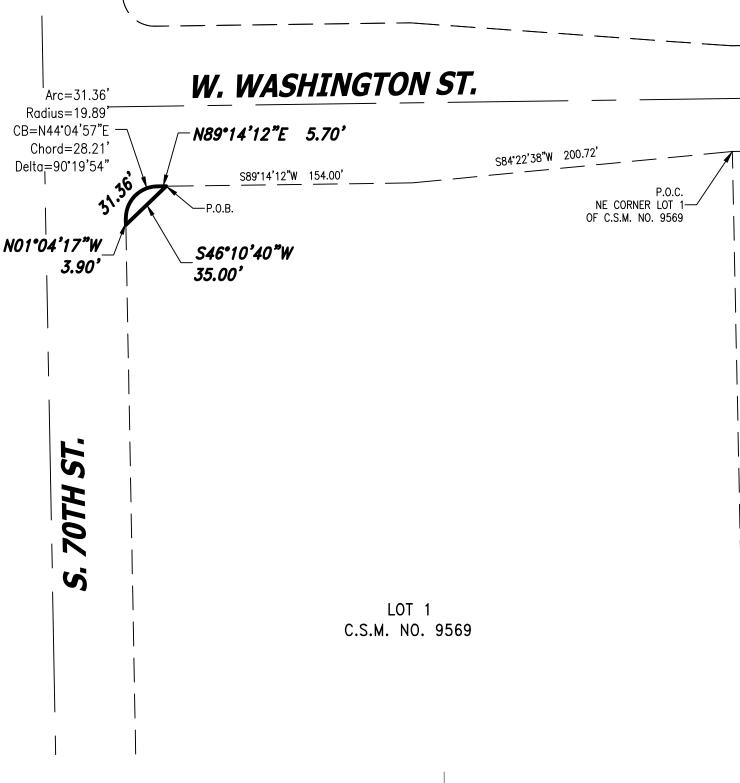
Bearings are referenced to grid North of the Wisconsin State Plane Coordinate System, South Zone (NAD83/2011), in which the East line of the Southwest 1/4 of Section 34, Town 7 North, Range 21 East, bears N01°01'28"W.
